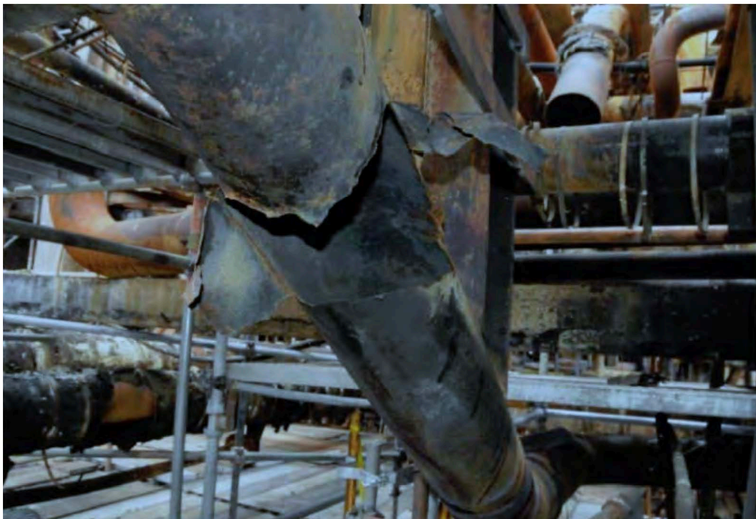
The August 6, 2012 fire at the Chevron oil refinery in Richmond, California, began near the rupture in this 8" pipe, shown in a photo included in the U.S. Chemical Safety Board's final investigative report. Credit: U.S. Chemical Safety Board
