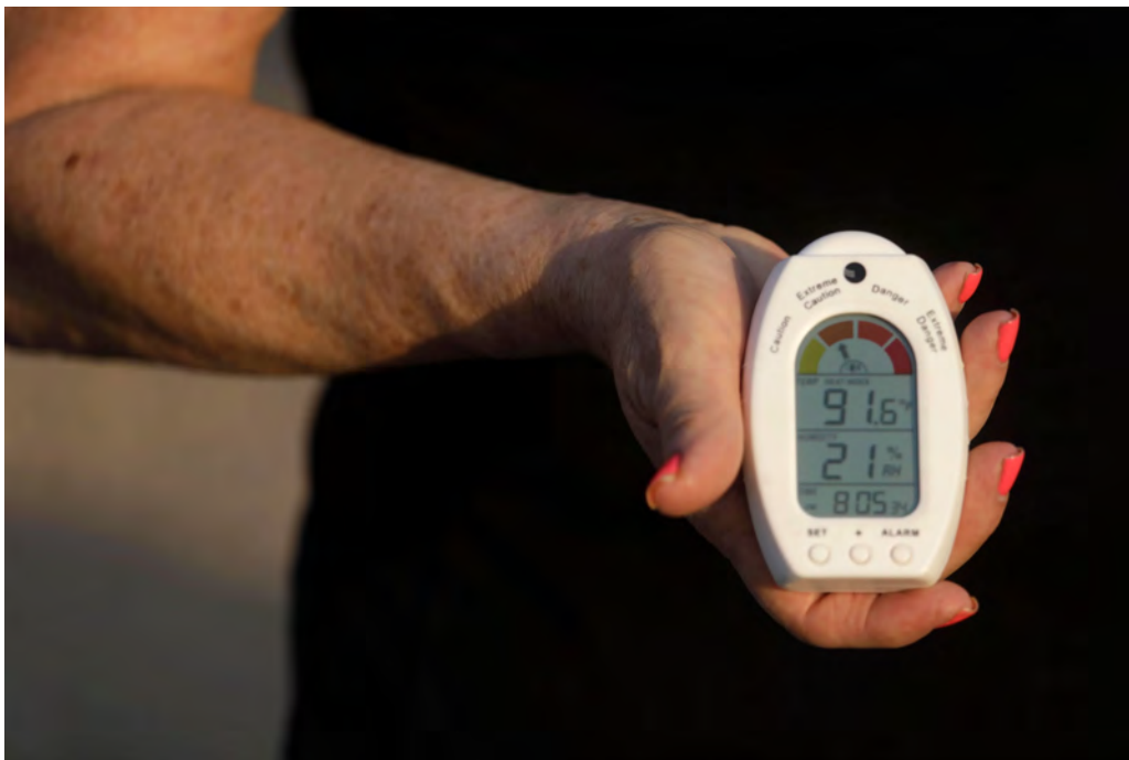
Debbie Fontaine holds a heat and humidity index device that some workers wear when working at the Rite Aid warehouse in Lancaster, California, on July 11, 2021. Workers have to take a break if the device reaches 90 degrees. (GENARO MOLINA/LOS ANGELES TIMES VIA GETTY IMAGES)
